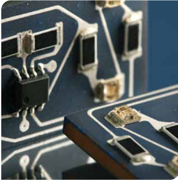
Close up of space saving surface traces and components on a rectangular CapStrate®
