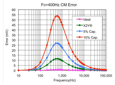
Figure 6: Output error voltage for various component mismatches
