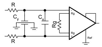
Figure 8: Added differential filter capacitor C<sub>x</sub>
