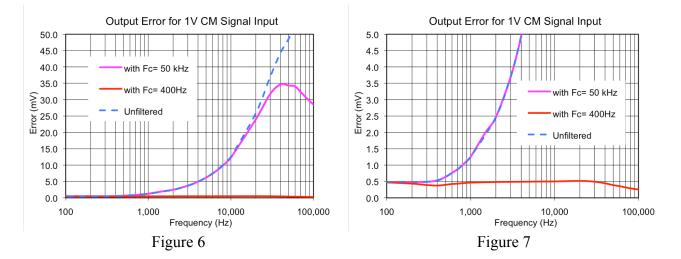
Adding the CMR optimized input stage filter has increased the effective common-mode rejection range by over two frequency decades limiting the CM error signal to just 0.5 mV. The trade-off is a reduction in system bandwidth. If additional bandwidth is required, setting the input filter pole frequency to 1kHz would limit CMR noise to 1.5mV and a 4kHz filter would hold CMR noise to 5mV.
