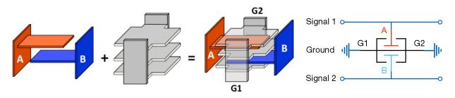
Figure 7: X2Y<sup>®</sup> capacitor construction with new symbol.
