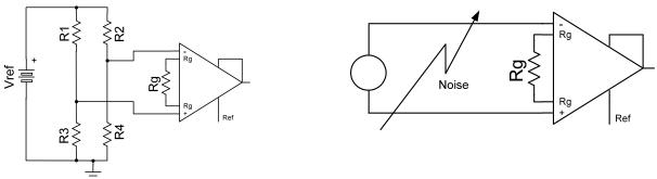
Figure 1: Common-mode voltage source
