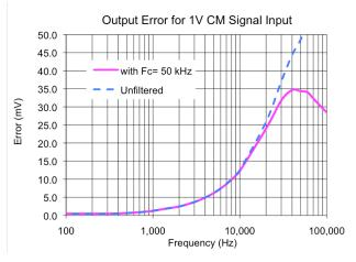
Figure 5: Output error with and without input filter
