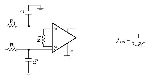
Figure 4: Single pole low pass input filters
