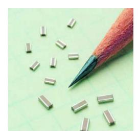
LICC capacitors are specially designed to exhibit lower inductance by altering the aspect ratio of the terminations. The smaller current loop length results in Equivalent Series Inductance (ESL) that is typically 60% lower then standard MLCs of the same size. This ESL improvement is extremely advantageous in the high frequency power decoupling of high speed digital MPU, FPGA, DSP, etc..
